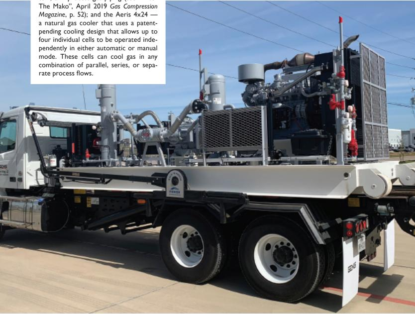
The G225 LE "Mako" is set to ship to its final destination on the back of the Genis roll-off truck. The Mako is a 225-hp (167-kW), 3-stage, wellhead compressor package that utilizes the same patent-pending cooling technology found on the Aeris cooler.
